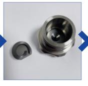
Place the orifice disc, plain bore facing downwards, on top of the O-ring.
