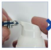
Assemble middle sized O-ring onto the retainer and apply a "dot" of grease to the circumference.
