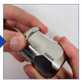
Hand tight only, screw down the nozzle body until it bottoms in the adaptor. There should be a "paper" thin visible gap between the adaptor and underside of the body.
