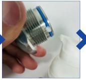
Apply a "dot" of grease to the circumference of the seal.
