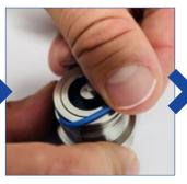
Now assemble the largest O-ring onto the nozzle body.
