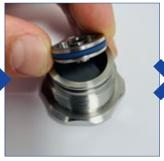
Insert the retainer disc into the body ensuring the raised profile sits on the back of the swirl chamber.
