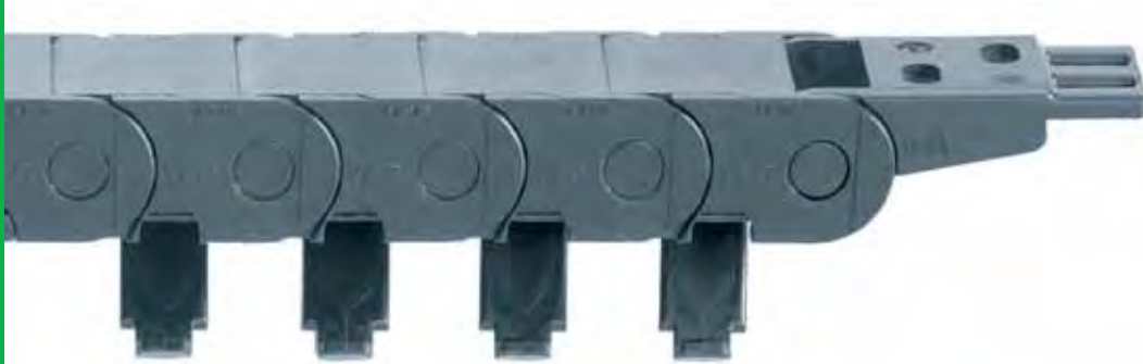
Series 14 | One-piece, snap-open along inner radius with film-hinge
