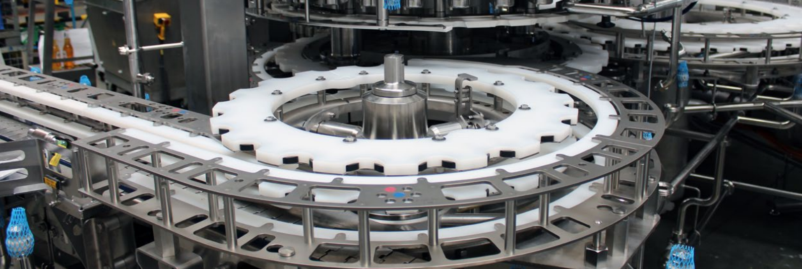
Injection-moulded clamping star wheels in Krones bottlers save setup times
