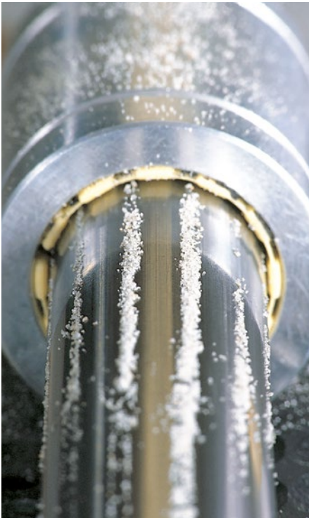
High wear resistance: plain bearing in permanent contact with sand
