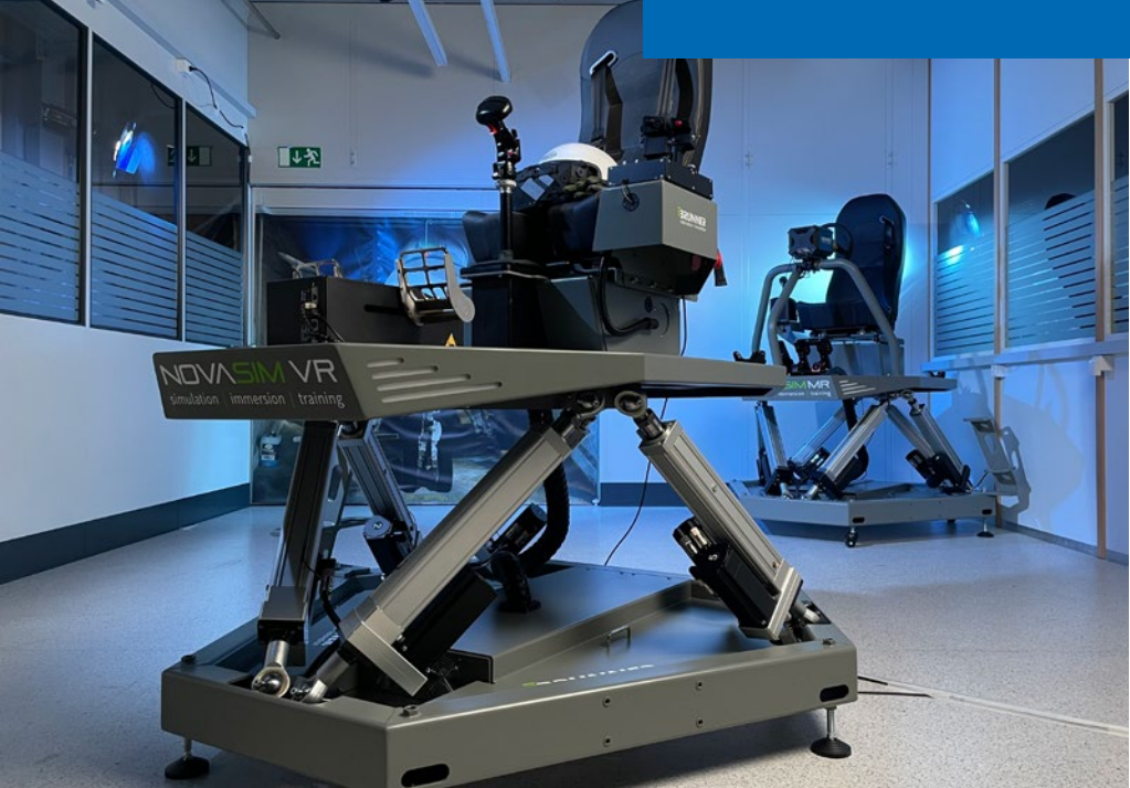
Precise adjustment for flight simulation of helicopters, jets, drones, etc., with the help of zero-backlash lead screw nuts
