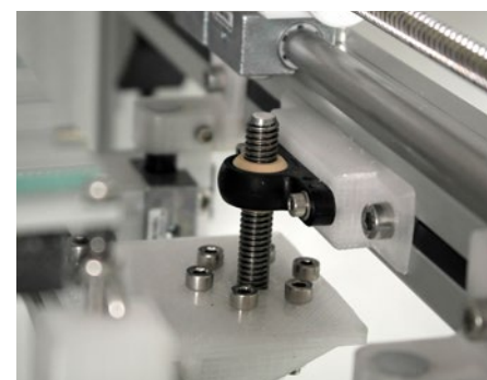
Spherical equalisation despite linear movement
