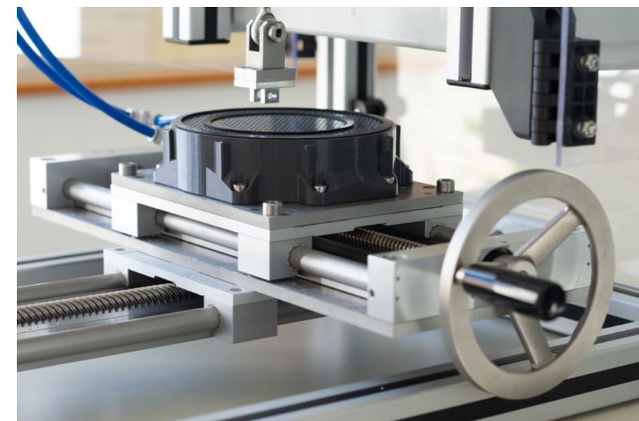
Linear module with dryspin® lead screw in a special measuring setup from Art Robotics
