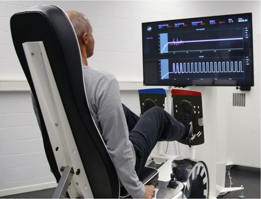
The core of the soft-robotic training robot is a pneumatic muscle, which generates this variable force and dynamics on the two pedals
