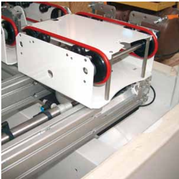
Handling and conveyance system for semiconductor transport/box.
