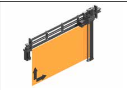
Workspace of a line robot in two-dimensional space
