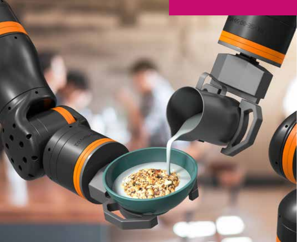
Ideal for service robotics: plastic robots with up to six degrees of freedom
