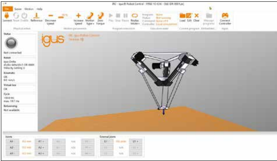
In the digital interface, the robot moves synchronously to the real robot
