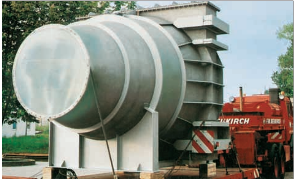
Droplet separator in a stainless steel housing
