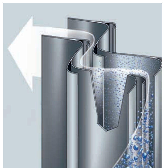
Functional principle of a horizontal separator
