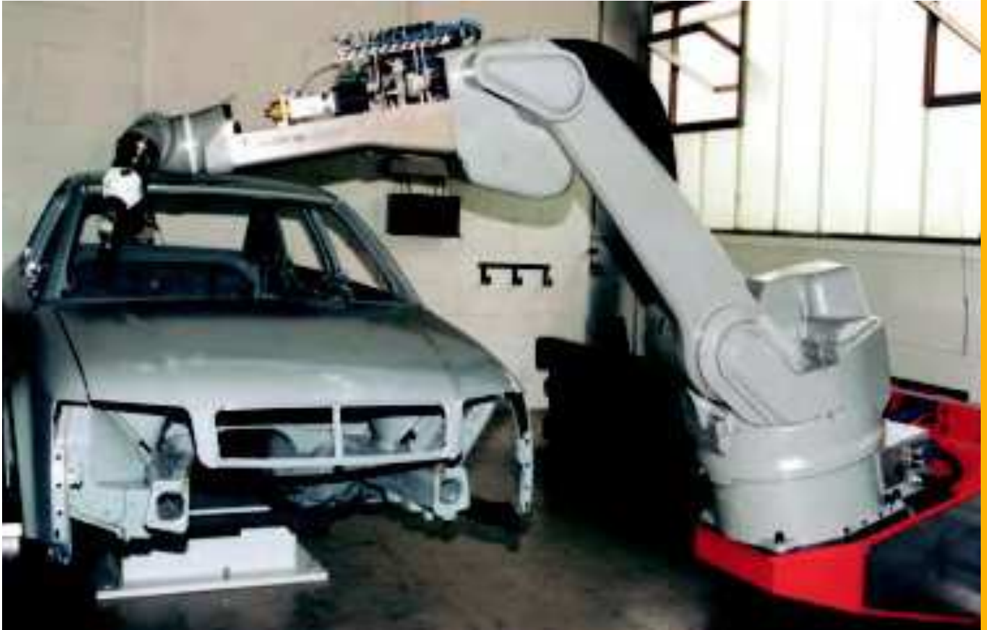
Spray-painting robot with System E4 e-chain® used in an ATEX version made of igumid ESD. High accelerations of up to 6 \text{ m/s}^2 and high braking rates with a weight of the robot of approx. one ton
